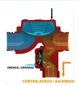
During the filter washing, the upper chamber closes and the lower one opens to invert the water flow, evacuating the dirt that the filter has retained.
