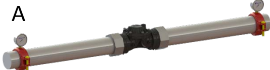
Friction Head Loss is measured from A to B.
