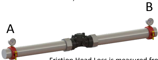
Friction Head Loss is measured from A to B.
